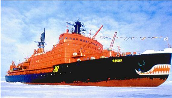
Route as well as in submitting a claim to a large part of the Arctic by the 2013 deadline. The largest part of the Russian icebreaker fleet is the nuclear powered *Arktika* class, built over a period of twenty years. They are the largest icebreakers in service anywhere, though Russia has announced plans to build even bigger vessels. The picture at the left is of *Yamal*, an *Arktika* class ship.
